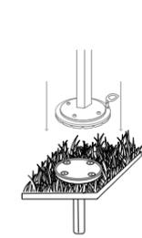
CONCRETE ANCHORAGE FOR ROTATION SUPPORT\*
