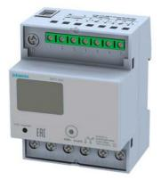
E counter with LC display, 3-phase, 80 A, 2xS0, 2 tariffs, Direct connection with meter zero setting data transmission function  $\,$
