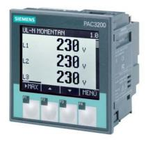
SENTRON, measuring device, 7KM PAC3200, LCD, L-L: 690 V, L-N: 400 V, 5 A, 3-phase, Modbus TCP, optional Modbus RTU / PROFINET / PROFIBUS, apparent/ active/reactive energy, class 0.5 acc. to IEC61557-12 or class 0.5s acc. to IEC62053-22, wide-range pwr sup. unit AC/DC, screw terminals
