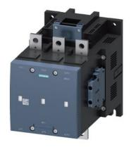
vacuum contactor, AC-3 400 A, 200 kW / 400 V AC (50-60 Hz) / DC operation 440-480 V AC/DC auxiliary contacts 2 NO + 2 NC 3-pole, frame size S12 busbar connections drive: conventional
