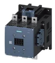
Contactor, AC-1, 690 A/690 V/40 °C, S12, 3-pole, 200-277 V AC/DC, PLC-IN optional, with varistor, 2 NO+2 NC, Connection rail/ screw terminal
