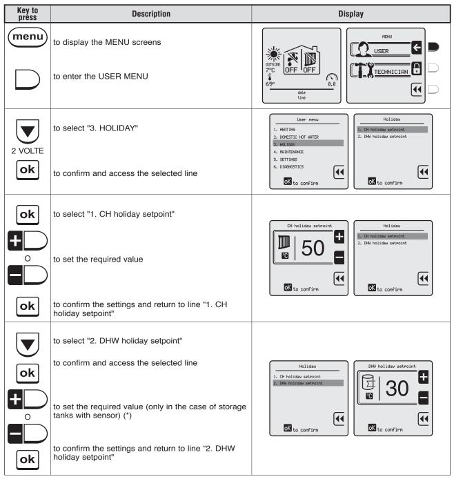
(\*) In the case of storage tanks with thermostat, take care not to set an excessively low value, as this could cause continuous requests for domestic hot water.
